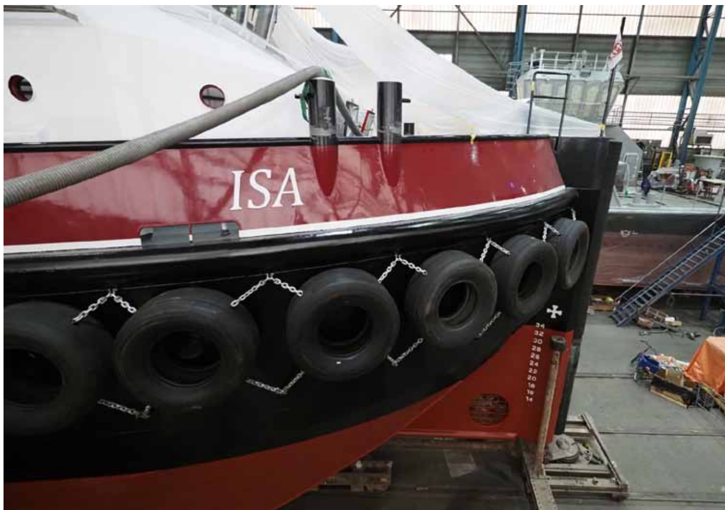
The "ISA", built in 2017, is a shallow draft anchor handling tug of 32,27 by 9,10 meters.
