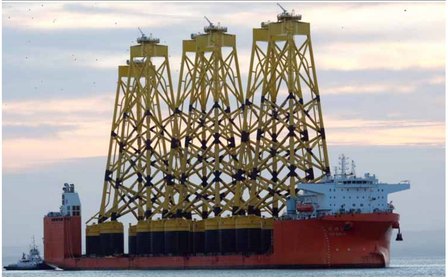
The 2019 built 240 Mtr x 48 Mtr FAN ZHOU 10 navigating the SUTORS of CROMARTY inbound PORT of NIGG with six Foundation Jackets onboard for the SEAGREEN OWF. The CALEDONIAN TOWAGE Tugs STRATHDEE STRATHDON and KINDEACE assisting. Photo : David Meek ©
